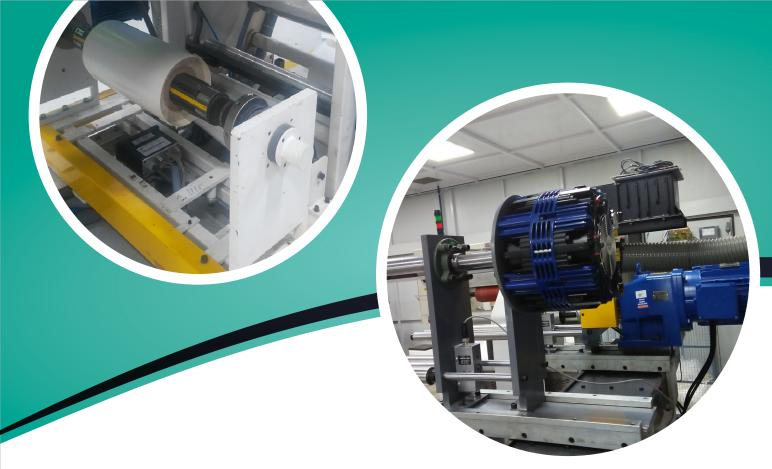
Our Unwinders and Rewinders guarantee the perfect stability on which the quality of the end product is based. Our winding and unwinding systems fit in any coating line, shaftless or with winding shafts, tension control in automatic mode throughout the diameter and operate with the same high precision from 0.1 m/min to 500 m/min. The winders can be used for a wide range:
